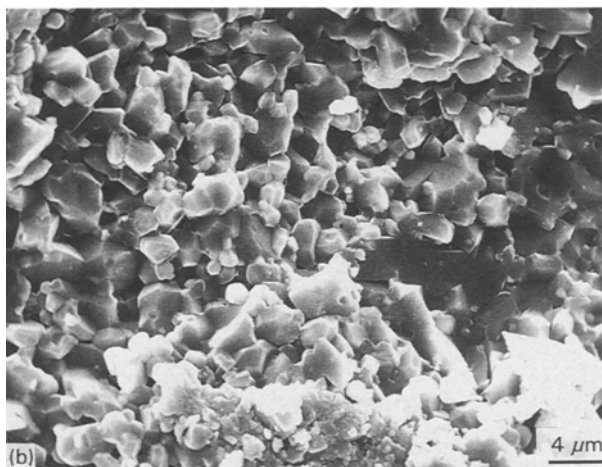
Figure 2 Scanning electron micrographs of (a) 7 GPa and (b) 10 GPa shock-treated and air-sintered \text{Al}_2\text{O}_3 -5 vol% \text{ZrO}_2 composites exhibiting local grain growth at the interior of agglomerates shown in Fig. 1.
